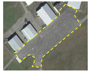
The construction activity will be phased to minimize impacts on airport operations. The construction phasing includes 3 work areas each with specific operational requirements. The total contract time is 80 Calendar Days. During this time, each of the apron and hangar entrances will be closed to aircraft at various times to facilitate construction.
